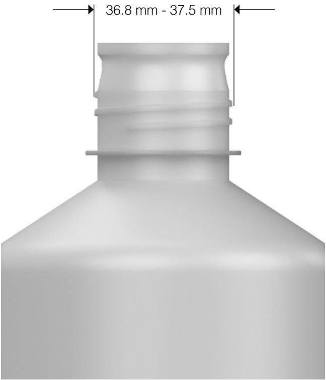
38-430 Nalgene plastic thread Scale 1:1
